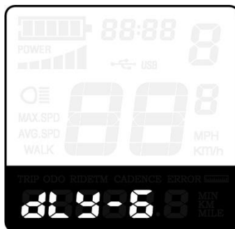
Delay Time of Battery Power Interface
