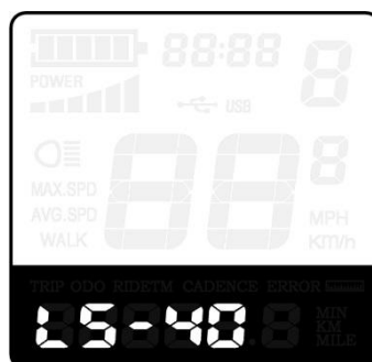
Interface of Max. Speed Limited Settings
